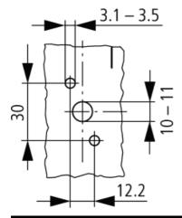
Diameter of drilled hole Door
